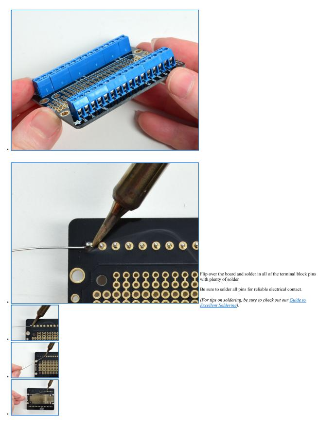
Check the first row once its done, to make sure each pin is shiny and completely soldered
