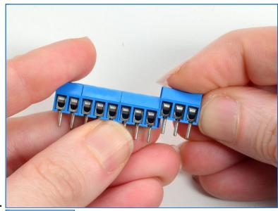
Keep sliding more 3-pin blocks on until you get a 2-pin block with four 3-pin blocks in the middle and then another 2-pin block at the end
