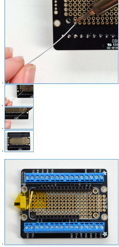
If you'd like to install the slide on/off switch, snap it into place at the end of the PCB and tape it down so it doesn't fall out when soldering
