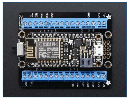
The terminal blocks allow you to connect to any of the external Feather pins, great for wiring temporary or permanent installations. We also give you a few extra terminal block pins for ground and 3.3V connections since those are so useful.
