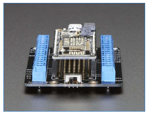
Comes as a kit with a nice PCB, socket headers, terminal blocks, and a slide switch. Soldering is required to assemble the Terminal Block Breakout FeatherWing, but it's not too tough if you've got a soldering iron and some basic hand tools.
