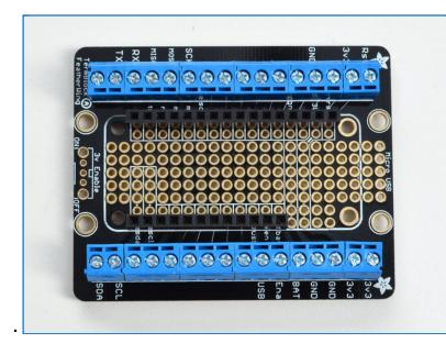
Next up place the 12-pin and 16-pin headers in the center part of the breakout in the outer-most set of holes
