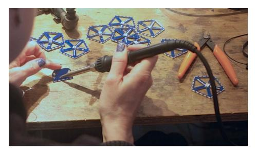
Then just solder in place. See how the back of the PCB is blank here? Make sure you can't see the lettering.
