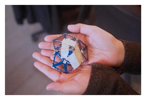
Now we're going to start soldering the BlinkyTiles together. The easiest way to do this is to tape the first three tiles together at the correct angle, like this.
