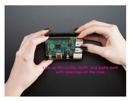
Here's how to insert a Raspberry Pi into our case:
