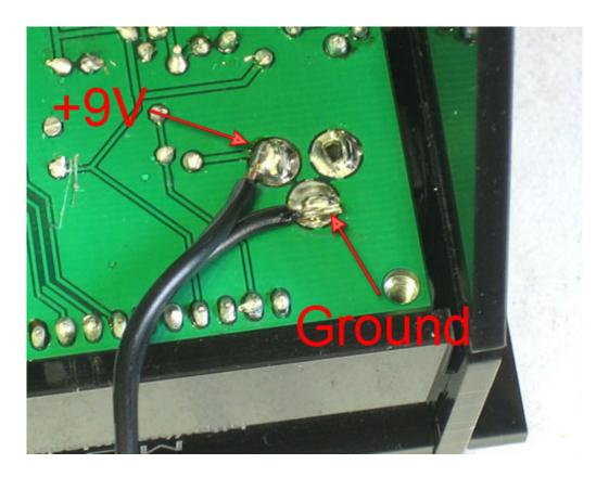
Now remove the bottom of the case (with the printing) and start sliding the back on, adjusting the cable as necessary.
