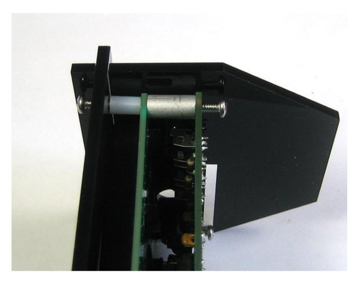
Annoyingly, the display has holes that are just a tiny bit too small for 4-40s, so you may find theres some resistance to screwing the front on. Just don't keep pushing hard after the screw gets to be flush with the front.
