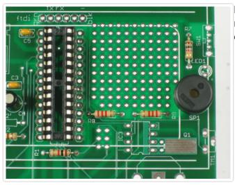
Place the piezo beeper **SPK**. This is the alarm noise-maker! It is non-polarized and can go in either way.
