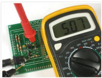
Now we are ready to do our first test. Clear off your table and make sure there are no wires or bits that could short out the PCB.
