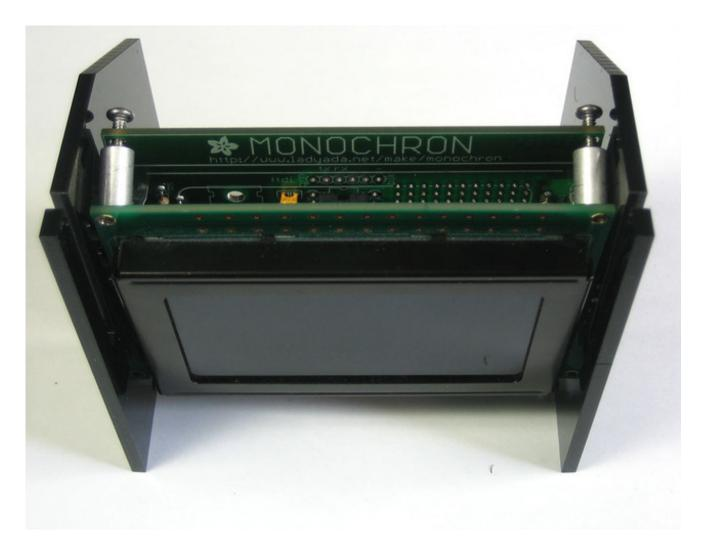
Now (perhaps with help from a friend if this is difficult) slide the front down onto the sides.
