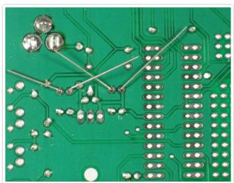
Once the electrolytic capacitors are placed correctly, bend out the leads and solder them in place.
