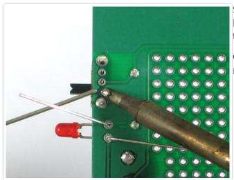
Solder in the LED and switch, watch out because the switch has some smaller pins in the middle. Don't use tons of solder.
