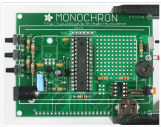
Now that the RTC is done, we will solder in the 3 interface switches **S1**, **S2**, and **S3**. These are what allow you to set the time and alarm and date and all that great stuff. They will snap into place, try to get them as flat to the PCB as possible.
