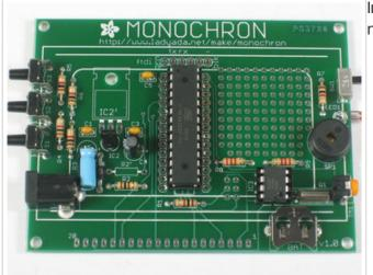
Insert the DS1307 RTC chip into the socket, making sure to align the U notches.
