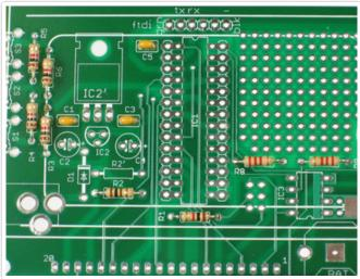
Now that we are done with the resistors it's time to solder in the ceramic capacitors.
