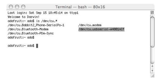
The name we are looking for is /dev/cu.usbserial-XXXX where the X's are going to be unique for each cable. Copy and paste the name into a text file so you'll remember it for later.
