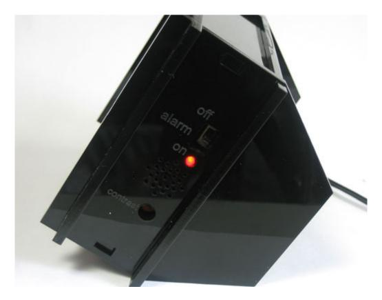
If the alarm is going off, the piezo will beep loudly and the display will flash. You can turn off the alarm by flipping the alarm switch on the side.
