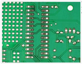
You can keep the socket in place with tape or if you have long fingernails, by bending over two of the little legs to hold it in place.
