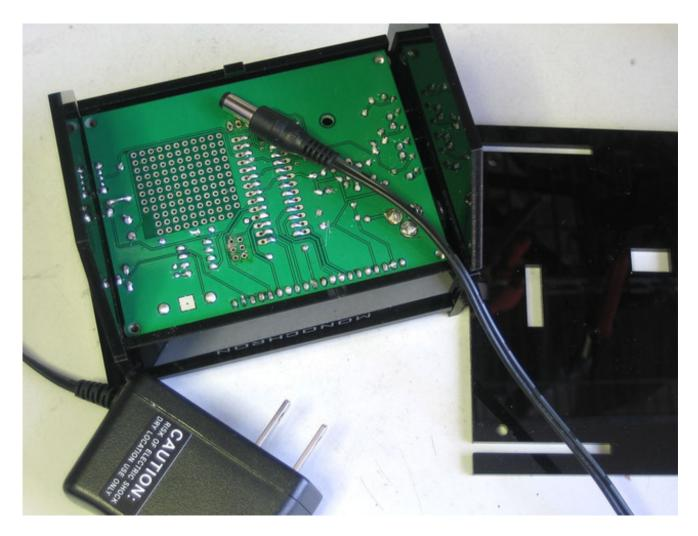
Cut off the end of the power supply. Of course, it shouldn't be plugged in at this time!
