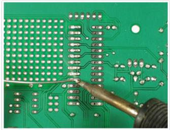
First solder in 2 opposite corners. Then solder the rest of the pins.
