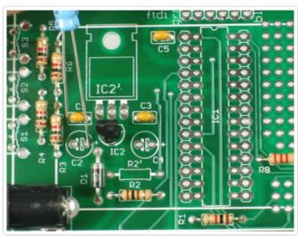
Now we will solder in the two electrolytic capacitors **C2** and **C4**.
