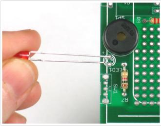
Now it's time to place the small indicator LED **LED1**. LED's are not symmetric and must be placed correctly in order to work. You'll notice one leg of the LED is longer than the other. This is the *positive* leg. The positive leg goes into the hole with a + next to it. In the picture shown, it's the left hole.
