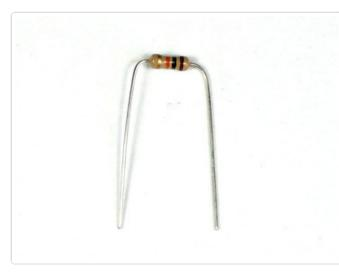
OK! Lets start! First thing we will solder in is the resistor **R1**, which has a 1Kohm value. You can tell which one this is because it has Brown Black Red Gold stripes on it. Bend this resistor into a staple as shown. Then slip it into the spot in the lower middle, right over the matching silkscreen that is labeled **R1**. Resistors are not 'polarized' so you can place them either way and they work the same. The resistor should sit right up against the PCB.
