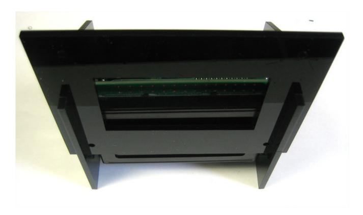
Once the front is in place, grab a spacer with pliers, and hold it between the case front and PCB while you feed in a machine screw to keep it in place.
