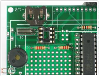
Now place the 8-pin socket (watch the U-tab) and 32.768 KHz watch crystal **Q1**. The socket is to protect the chip and the crystal is the same as whats in your watch or clocks.
