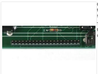
Once the female header is solidly in place, slip the male header into the sockets so that the short pins stick up.
