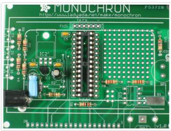
Now place the IC socket. The socket protects the microcontroller chip and allows it to be replaced if necessary.
