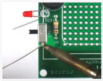
You may want to tack solder the switch from above to keep it in place. Make sure the switch is sitting flat against the PCB.
