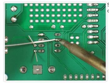
Solder the socket and crystal, then clip the crystal leads.
