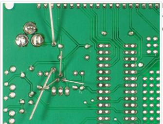
Now flip over the PCB and solder in the diode and regulator.
