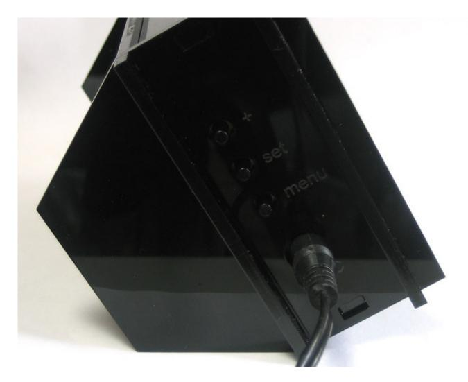
There are three buttons, **MENU**, **SET**, and **+** for configuring the clock, snoozing and displaying the date.
