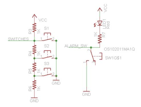
There are 2 sets of switches, the configuration tactile buttons and the alarm switch. The alarm switch is simply to indicate whether the alarm is on or off. To save a pin, the indicator LED (**LED1**) is connected directly to the switch paddle through a current limiting resistor **R7**.
