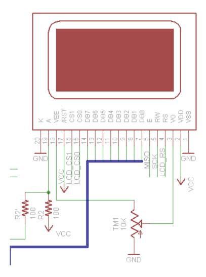
The main display is a monochrome **KS0108** based LCD with 128x64 pixels (two 64x64 pixel controllers) It is a well known and documented display. They are common in electronics shops, and run at 5V. The unfortunate thing about them is they're quite sluggish and so they need software optimization for any sort of animation.
