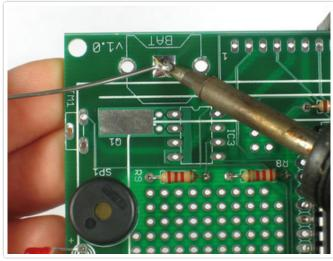
Now we will solder up the real time clock (RTC) circuit. The RTC is what keeps time when the power is out, it's a very very very low power microcontroller and crystal that will keep time for years on a tiny coin cell. This way you can mod your clock with ease and not have to reset it after power loss.
