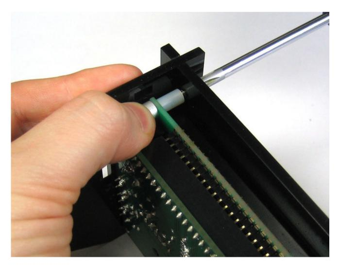
Once the screw is sitting flush, stop. Don't force it or the acrylic could crack.
