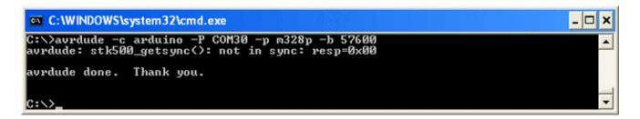
Check that you have the cable in properly and you're holding it right. Then press the up arrow and return to try again.
