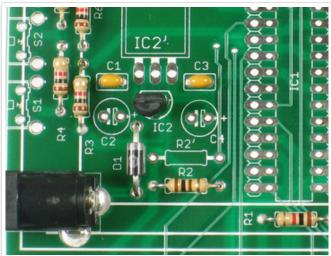
After the diode is the 7805 voltage regulator **IC2**. The 7805 regulators up to 17VDC down to a nice steady 5V. Because we are using a good quality LCD with an LED backlight, we don't need a big honking power supply chip. The TO-92 package 7805 can supply about 100mA.
