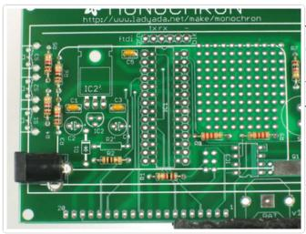
Now we are ready to build the power supply. The power supply is what takes 9V from the outside world (from power plug) and regulates it down to 5V that is safe for the microcontroller to run at.
