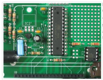
Place the female header strip with the sockets up in the PCB.
