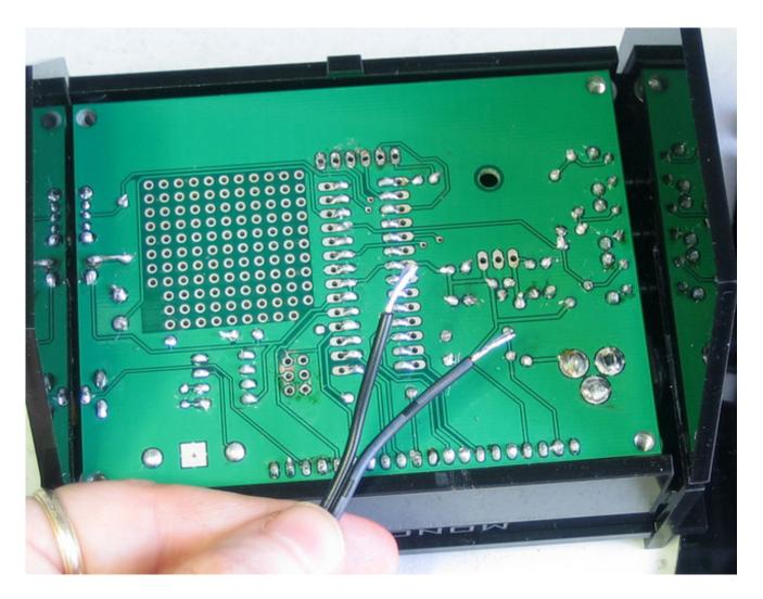
Use a multimeter to verify which wire is ground and which is +9V
