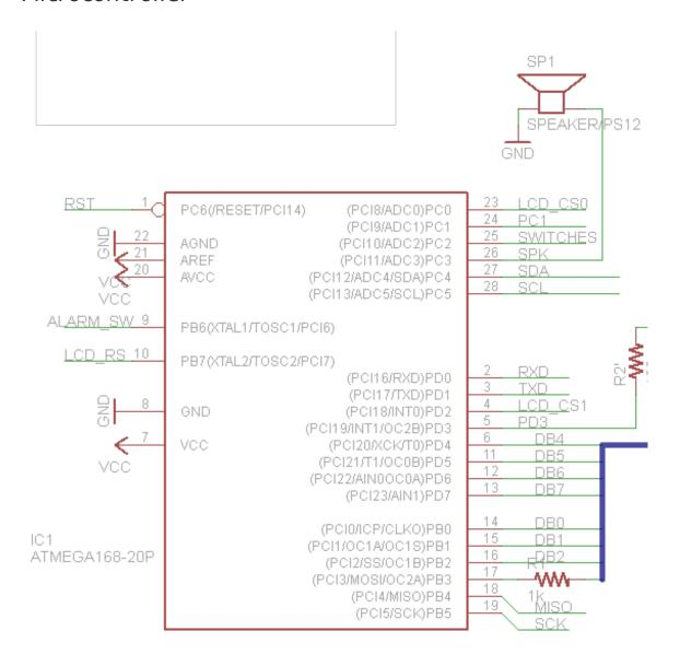
Finally we get to the microcontroller. The microcontroller does not have a crystal, we'll be running it using the internal 8MHz oscillator which is good enough, this frees up two pins. **R1** is used because otherwise the LCD output on that pin conflicts with programming (**MISO** and **SCK** go into an input pin on the LCD).
