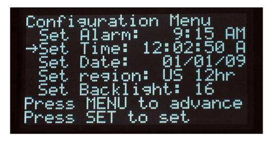
Press **SET** to start setting the time. Press + to increment the hours. When you're done, press **SET** to advance.
