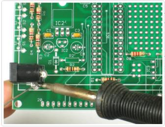
If it doesn't snap in place, you can keep it from falling out by 'tack' soldering it a little from the top on one of the pins.
