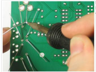
Flip over and solder the resistors just like before, making sure to heat each joint and fill it with solder completely.
