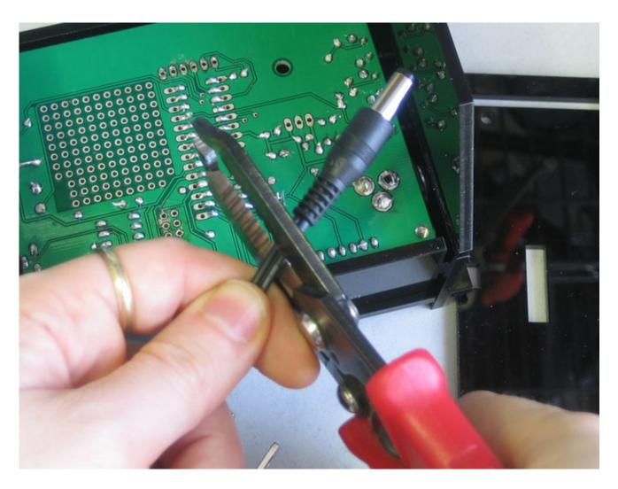
Pull the two wires apart, sometimes cutting with nippers helps you get started
