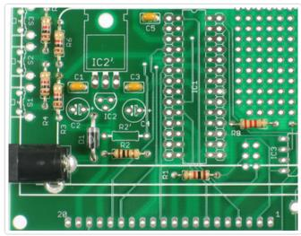
Next is **D1** the 1N4001 protection diode. Diodes are semiconductors, in particular a diode will only pass current in one direction. This protects the power supply and micro from if someone plugs in a power supply that is AC or negative polarity. Instead of going poof, the diode will block the negative voltage.
