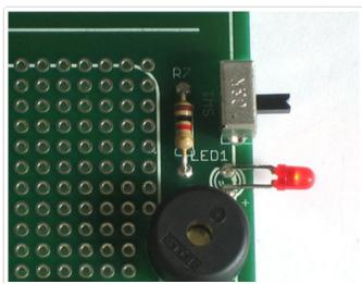
Now you can do a test of the LED and switch if you'd like. Clear off your desk and power up the clock. It will still beep, but now you can flip the switch back and forth and see the LED turn on and off!
