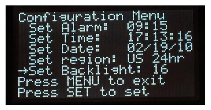
Press + to cycle through the brightness, from 00 to 16. You may have to adjust the contrast at the same time to get the ideal display!
