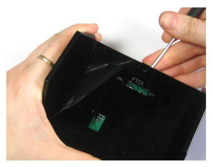
Screw on the 4 remaining bolts to keep the kit together! Don't overtighten, just tighen until the screws wont come loose.
