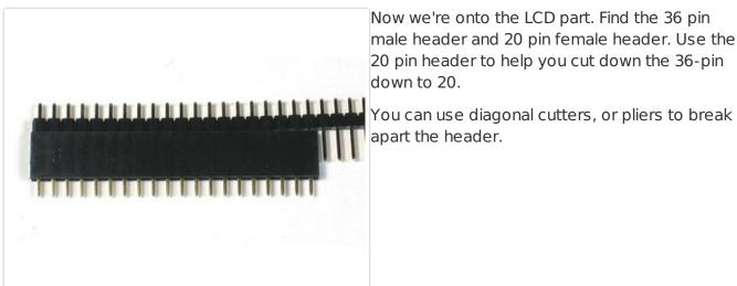
Now we're onto the LCD part. Find the 36 pin male header and 20 pin female header. Use the 20 pin header to help you cut down the 36-pin down to 20.
