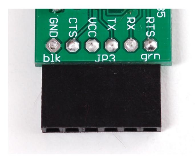
Stick a piece of 6 pin header left over from the kit making into the socket so that the shorter pins stick out. The latest kits come with an **extra long** header piece..use that!
