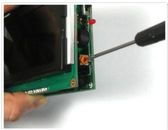
The trim pot on the side is used to adjust the contrast.
