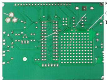
Flip over the PCB and solder in the resistors.
