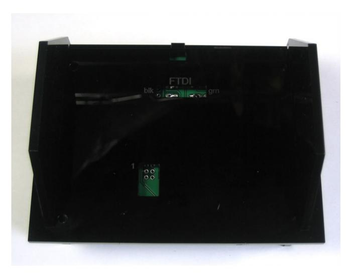
Finally, with a flathead screwdriver or similar, gently gently pry the back piece up while pushing it so that it snaps into place. Don't pry too hard, just enough to get the piece on.
