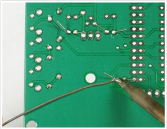
Flip over the board and solder in the 3 ceramic capacitors.
