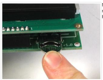
Now insert the coin cell, + side goes up. You must place the coin cell because otherwise the RTC will be erratic and the clock will act oddly.
