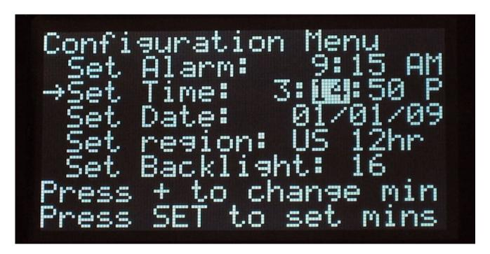
Press + to increment the seconds. When you're done, press **SET** to save the time.
