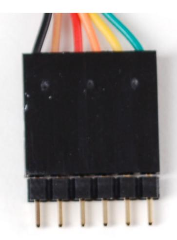
Now, plug in the header so that it fits into the back of the clock, so that the BLACK wire lines up with the text that says **blk** You will have to hold the cable so that you end up pressing the header at an angle against the socket, this way you will make contact without having to do any soldering.
