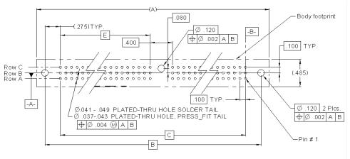
Recommended PCB hole mounting pattern
