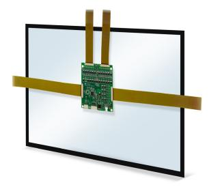
the active surface touch components. In addition to adding sophisticated industrial design, the flat front surface solution eliminates dust and debris build-up at the edges of the display and also helps increase overall system reliability by not having critical components on the touchscreen surface that can be damaged or obstructed.
