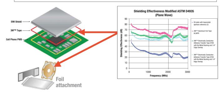
3M<sup>™</sup> Electrically Conductive Adhesive Transfer Tapes 9703, 9705, 9706, 9708, 9709, 9709S, 9709SL, 9712, 9713, 9714, 7805 and 7810 can provide FPC grounding and tapes 9708, 9709, 9709SL, 7805 and 7810 can increase the effective EMI Shielding through the bond line thickness leading to improved product EMI Shielding performance of the FPC.
