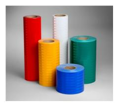
3M<sup>™</sup> Engineer Grade Prismatic Reflective Sheeting Series 3430 meets ASTM D4956 Type I and is a non-metalized, microprismatic lens reflective sheeting designed for production of non-critical traffic control signs, work zone devices and delineators that are exposed vertically in service.
