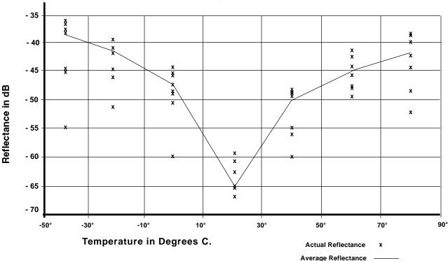
Notes: All splices were assembled with fiber cleave angles << 1 degree in order to maximize reflectances at the various operating temperatures.
