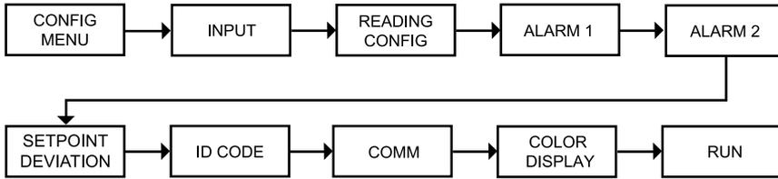
**Figure 3.2 Flow Chart for Configuration Menu**
