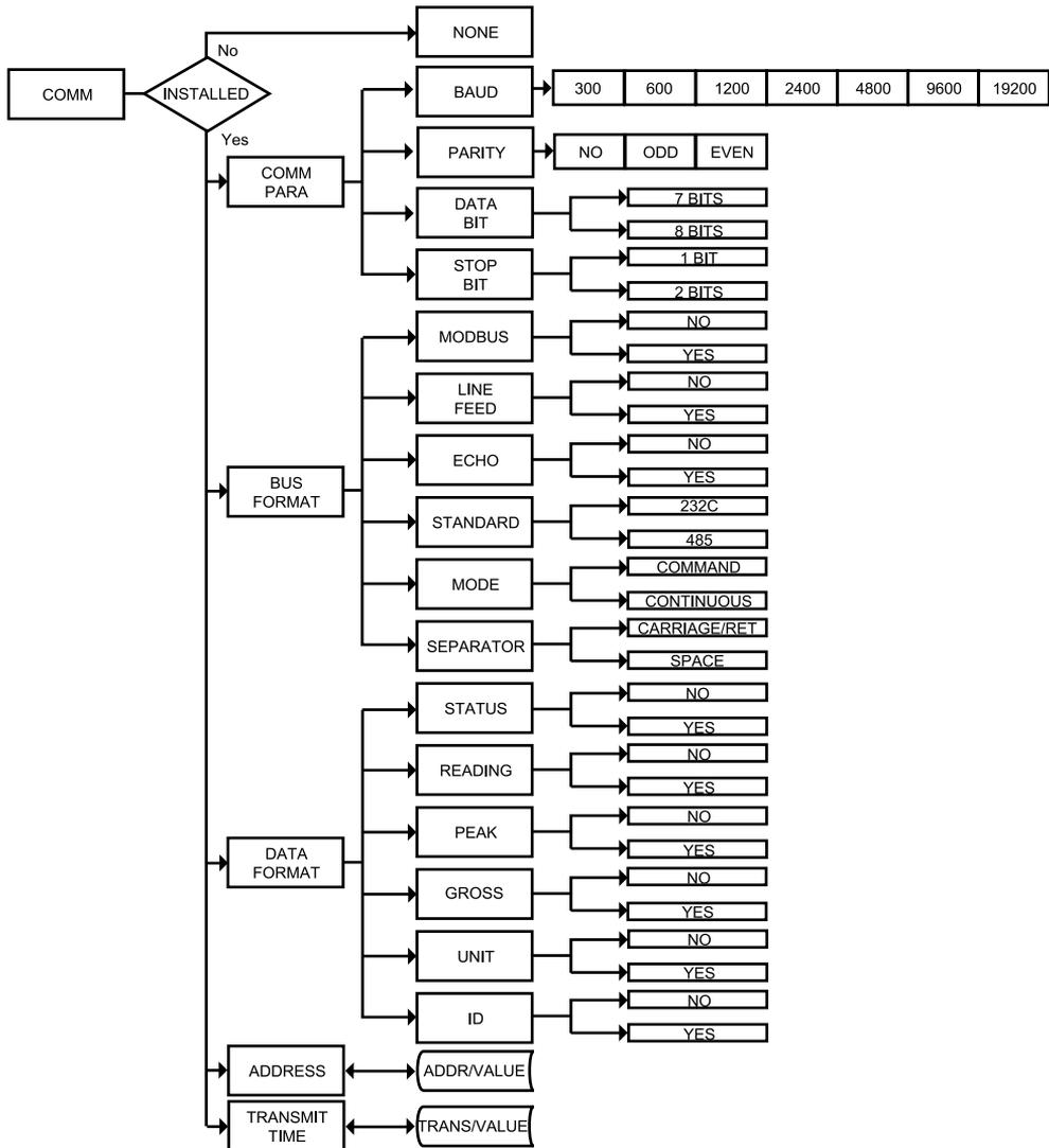
Figure 3.9 Flow Chart for Communication Option Menu
