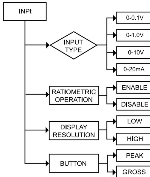
**Figure 3.3 Flow Chart for Input Type Menu**
