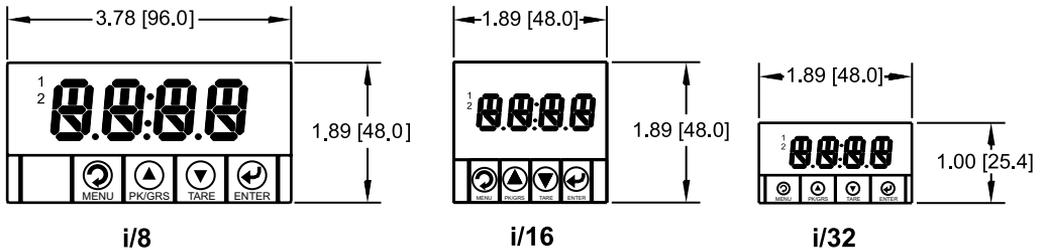
**Figure 2.1 Front Panel Display**
