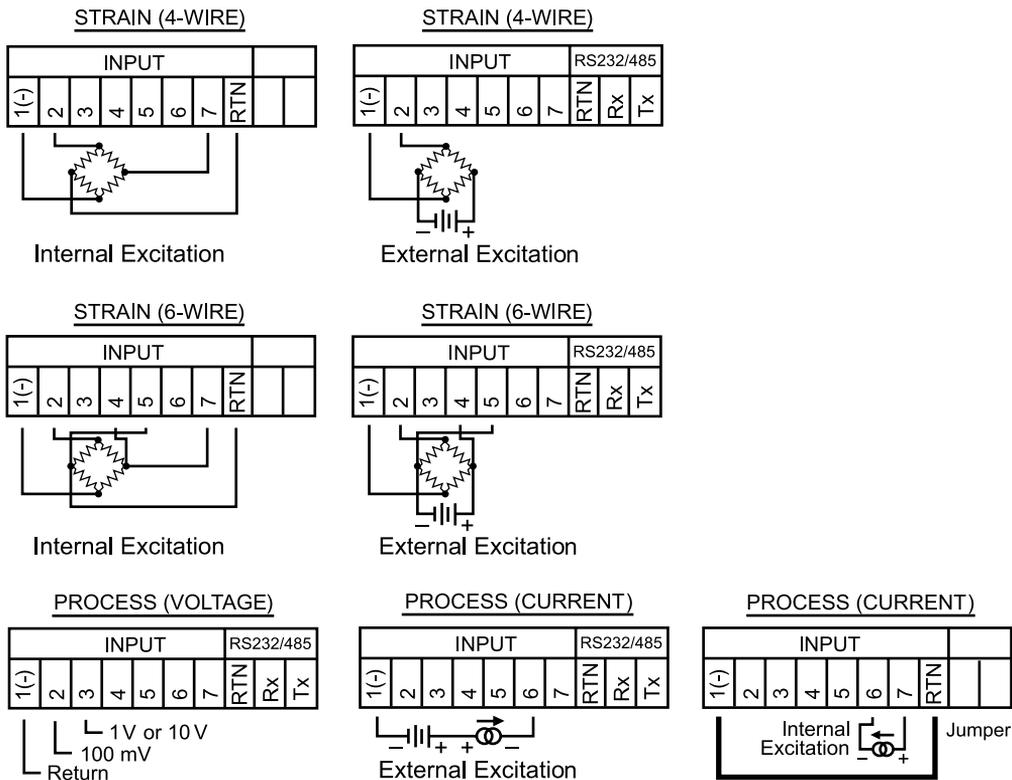
**Figure 2.3 Rear Panel Input Connections**
