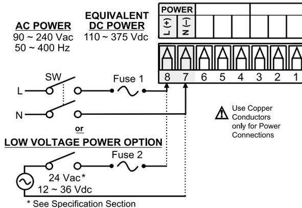
**Figure 2.4 Main Power Connections**
