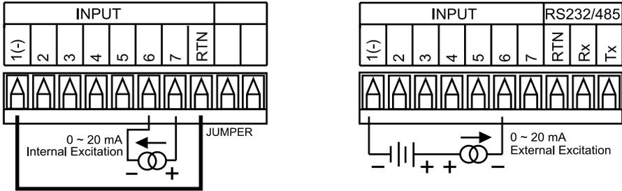
**Figure 2.5 Process Current Wiring Hookup (Internal and External Excitation)**
