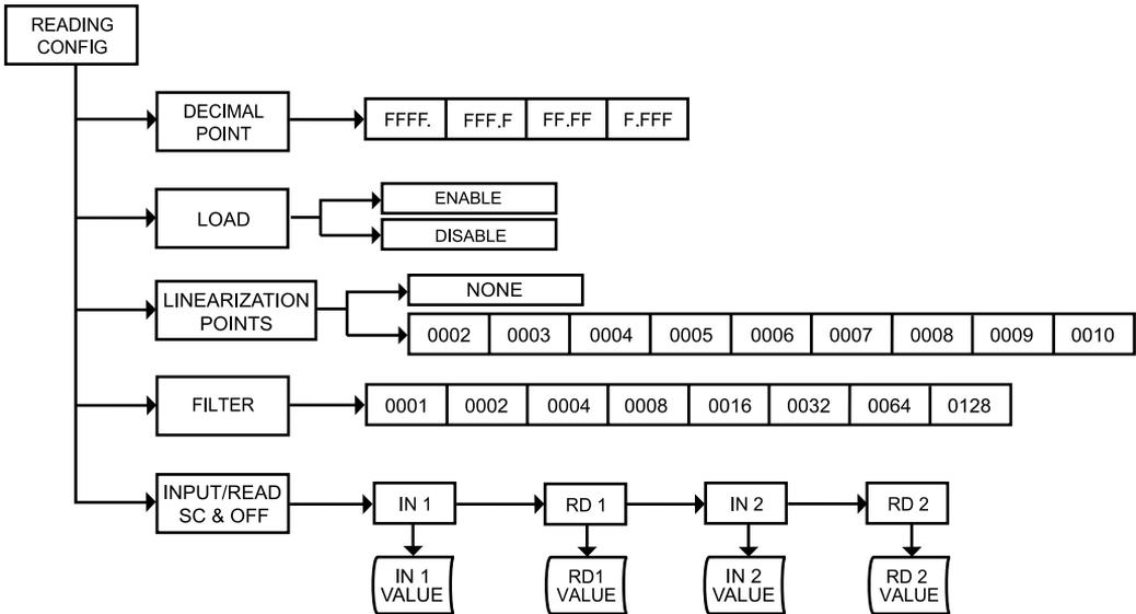
**Figure 3.4 Flow Chart for Reading Configuration Menu**
